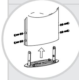
3. Secure the Mounting Bracket (**Part B**) by using the Bolts with washers that come pre-installed in the stakes.
