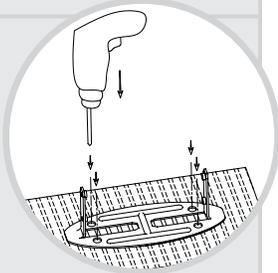
4. Insert the Concrete Anchors (**Part C**) into those holes and tighten them to the Mounting Bracket (**Part B**) using the Allen Wrench (**Part E**).
