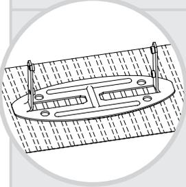
3. Drill four holes for the Anchor Bolts (**Part C**) using a drill. Each hole should be approximately 3/8" wide and 2.75" deep.
