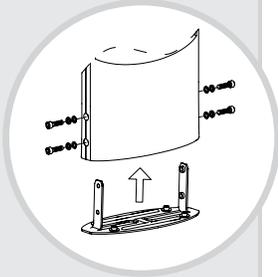
2. Place the Mounting Bracket (**Part B**) in the desired location of the lamp.
