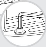
5. Slide the Solar Pillar (**Part A**) over the Mounting Bracket (**Part B**) and secure using the four screws (removed from the Pillar earlier) and the Allen Wrench (**Part E**).
