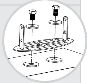
4. Slide the Solar Pillar (**Part A**) over the Mounting Bracket (**Part B**) and secure using the four screws (removed from the Pillar earlier) and the Allen Wrench (**Part E**).
