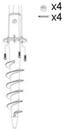
10.2 Use the Turning Bar (G) and Leveling Tool (in the EZ Anchor) to screw it in the ground as level as possible.
