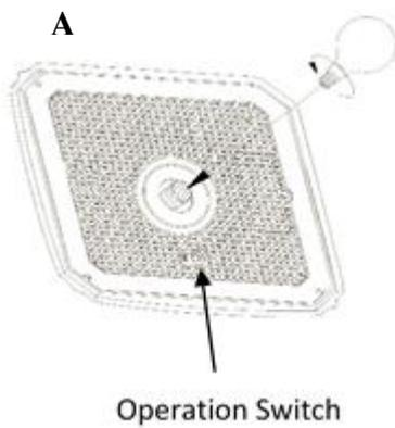
4. Attach top (A) to the body (B) with the two supplied screw caps.
